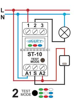
Fig. 4. Connection diagram of the STAIRCASE SWITCH in a 4-wire installation.
