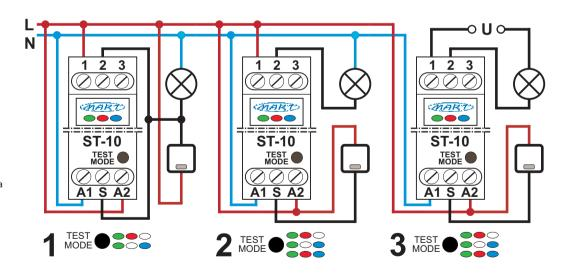
Fig. 1. Connection diagrams for the ST-10 STAIRCASE SWITCH automatic device.
