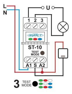
Fig. 5: Connection diagram of the STAIRCASE SWITCH in a 4-wire installation with an external power supply in the load circuit.
