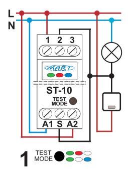
Fig. 3. Scheme of connecting the STAIRCASE SWITCH in a 3-wire installation.
